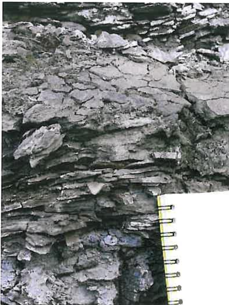
Photo 6. Closer view of the weathering of laminated sandstone of the Nanaimo Group.
