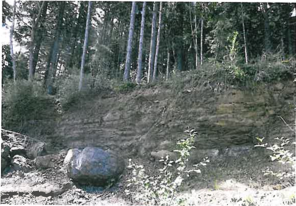
Photo 7. Borrow pit exposes thin veneer (<1m) of soils overlying Upper Triassic age volcanic bedrock of the Karmutsen Formation (Vancouver Group).
