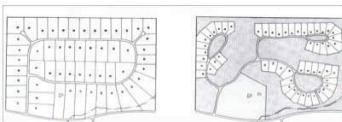
A typical conventional subdivision (left) and a clustered subdivision (right) with three clustered 'pods' of homes. At least 50% of the site is preserved as open space and the houses are clustered on slightly smaller lots. (source: http://www.pineplainsunited.org/density-zoning-vs-min-lot )
